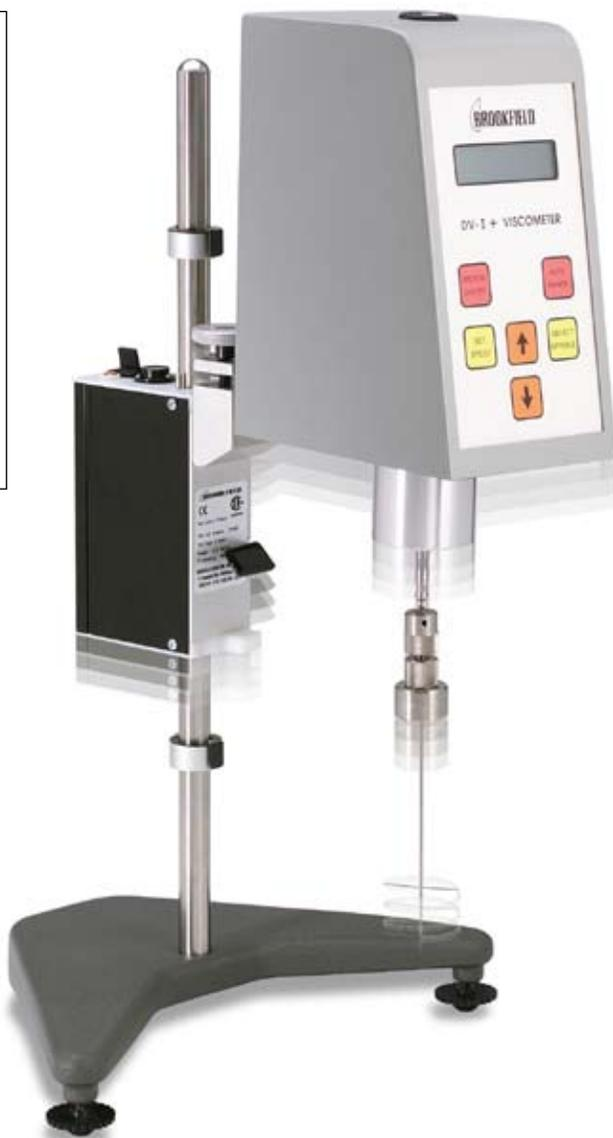
For viscosity/consistency measurement of gels, pastes, creams, putty, gelatin and other non-flowing substances.
