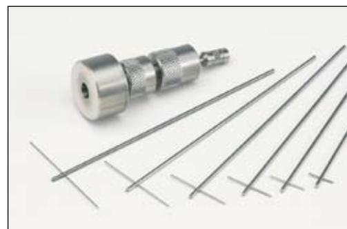
The Helipath Stand can be used with any standard Brookfield Viscometer model, and is supplied complete with a set of six T-bar spindles and a special coupling.
