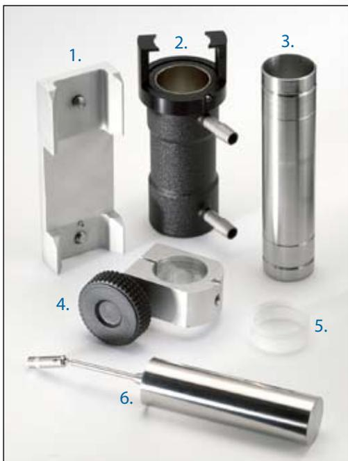
Detail of UL Adapter: 1. Locating Channel Assembly, 2. Water Jacket, 3. Chamber Tube, 4. Collar with thumbwheel, 5. Tube End Cap, 6. Spindle with universal coupling
