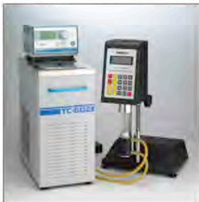
Figure 1: Chocolate Viscosity Test System includes Brookfield DV-III Ultra Rheometer with Small Sample Adapter and Temperature Bath
